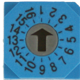
Figure 11: Rotary Switch Address Settings
