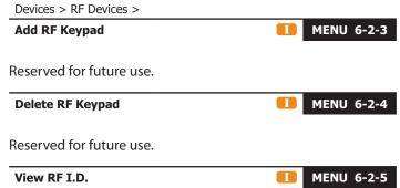
This command allows you to trap and view a transmitters I.D. number when it has been forgotten or it is no longer legible on the transmitter label. The device being tested must be compatible with the RF receiver fitted to the panel.
