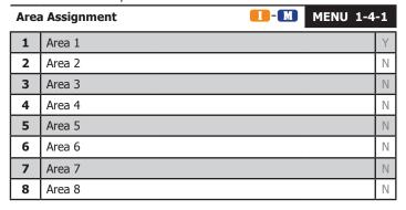
This menu allows the Installer or Master User to program which areas (1 to 8) other users can access. Each user can be assigned to one or multiple areas.
