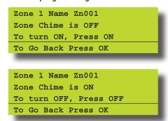
Press [ON] or [OFF] to toggle the zone to be monitored when Chime Mode is turned on then press [OK] to save and exit or [MENU] to exit without saving. Inputs > Commands >
