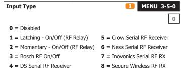
This menu option is used to configure the systems programmable input terminal. Various devices can be connected including keyswitches of radio controlled relays etc. When RF zones are required you need to connect the RF receiver to this input
