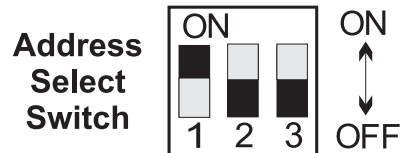
Figure 14: Keypad DIP Switch Address Settings
