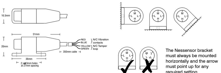
The Nessensor bracket must always be mounted horizontally and the arrow must point up for any required setting.
