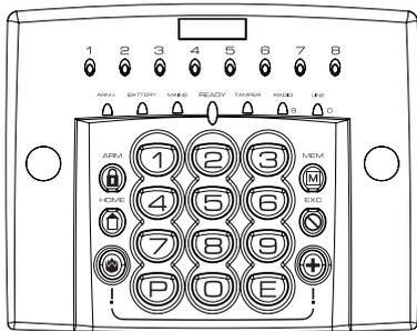
The Ness ECO8x keypad provides important visual and audible indication of the system status and is the main interface for controlling the many powerful features of the system.
