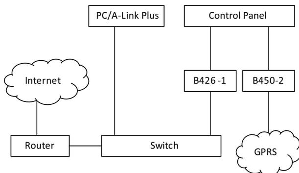
In the configuration diagram above, the control panel is programmed with Transmission Format as Email and two network modules are enabled to access mail server. It is an example of using B426/B426-M as network module 1 and B450/B450-M as network module 2. The wiring diagram is shown in above picture. “B426-1” means the rotary address switch of B426/B426-M is set to 1; “B450-2” means the rotary address switch of B450/B450-M is set to 2.
